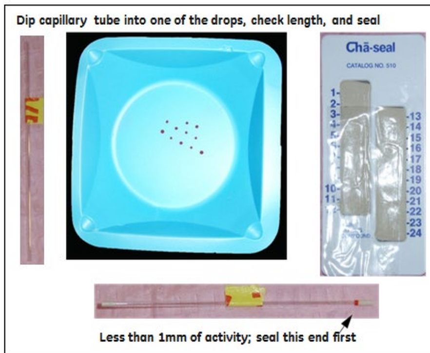
Figure 2.2: Fill and seal the capillary tubes
