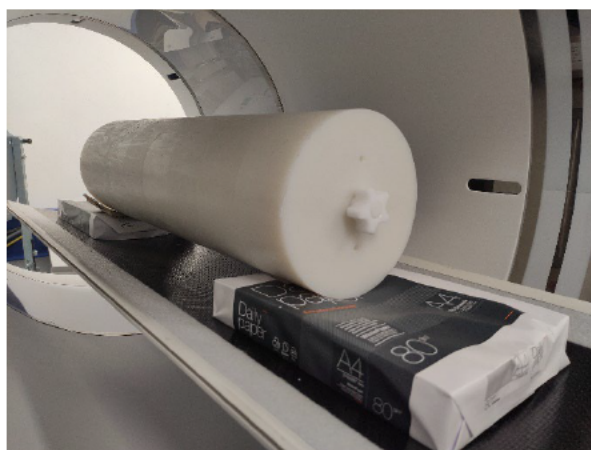
Figure 5.2: Line Source Orientation. Phantom shimmed on table.
